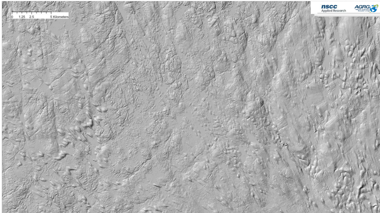
Figure 2 shows a lidar derived DEM of central south-western Nova Scotia (Springfield). Drumlin glacial till mounds are seen as topographic highs, whereas flat, possible wetland and water areas are visible as well. Lidar DEMs are typically shaded to accentuate surface features as is presented here.
