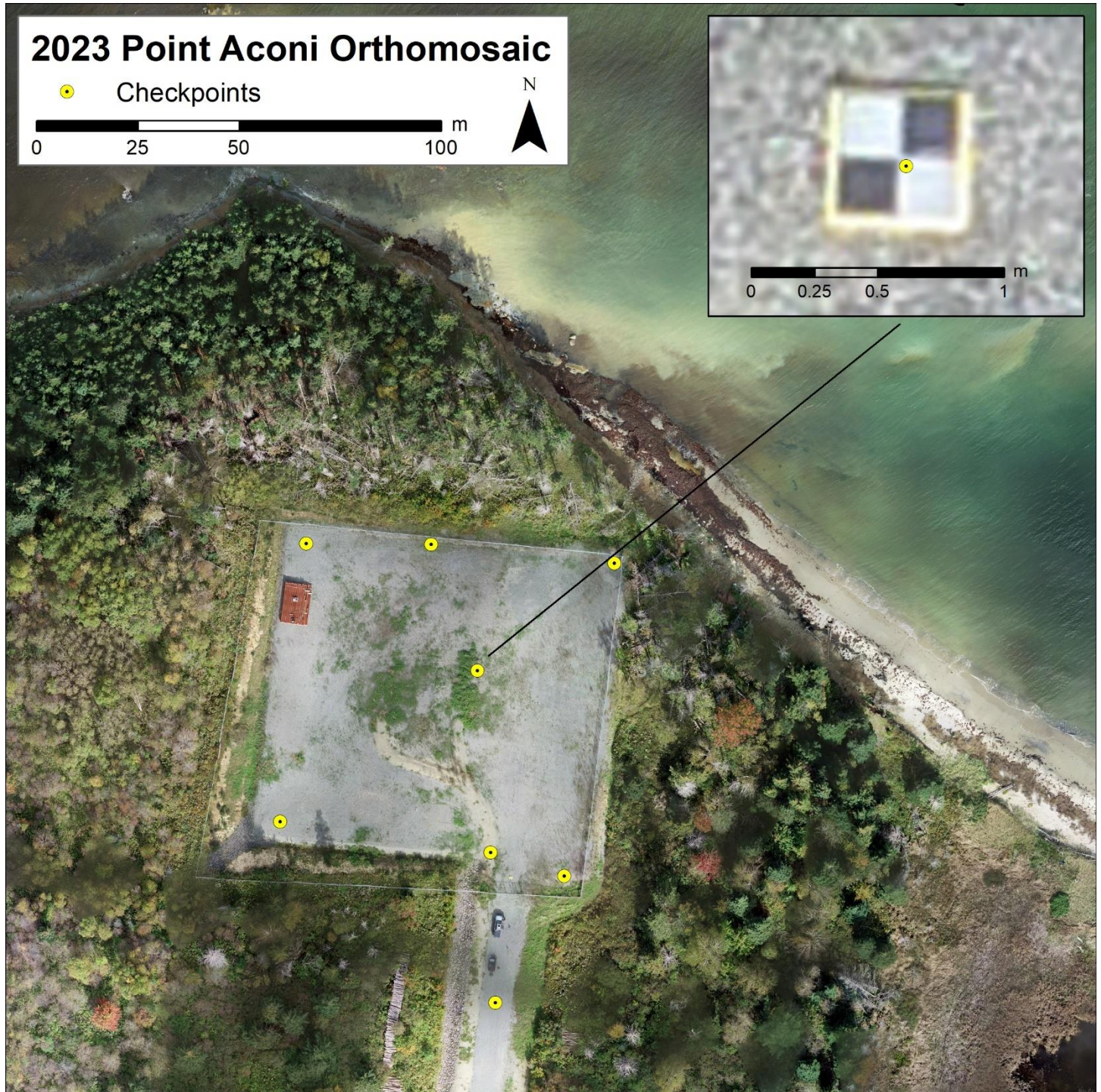
Figure 1. Point Aconi site photo mosaic showing good horizontal alignment over checkpoint targets.
