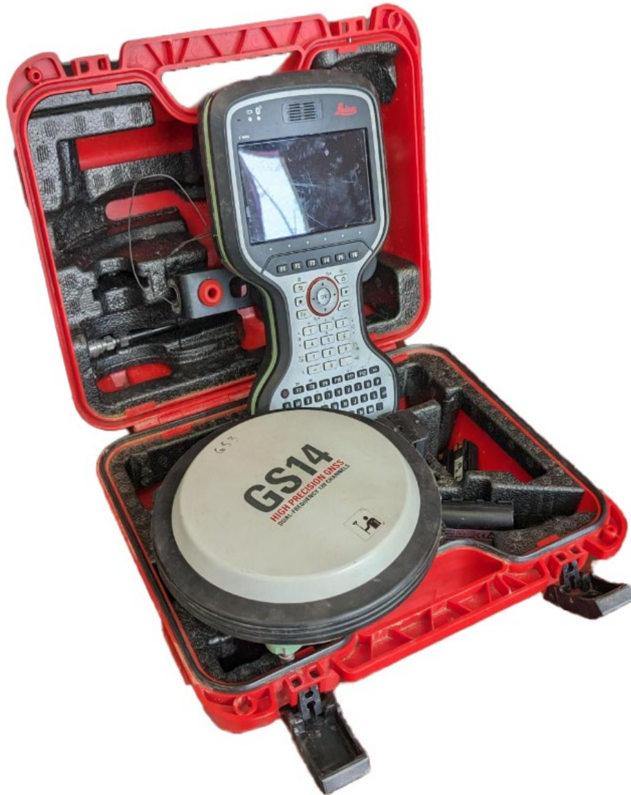
Figure 4. AGRG's Leica GNSS system, comprised of a GS14 antenna and CS20 controller. The antenna and controller are mounted to a pole in the field for data collection.
