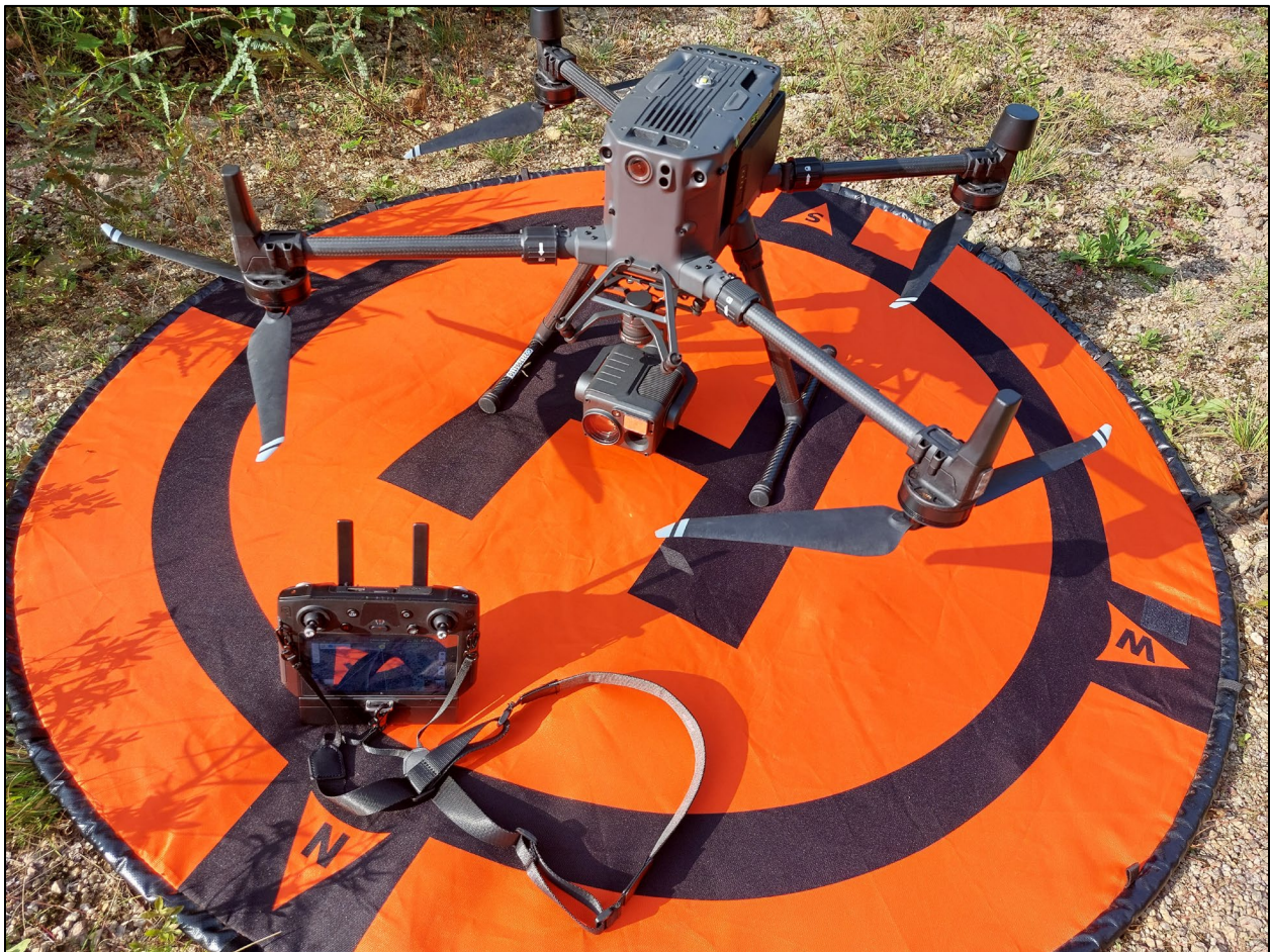
Figure. 3. AGRG's DJI M300 RTK RPAS with the H20T thermal/RGB sensor attached.
