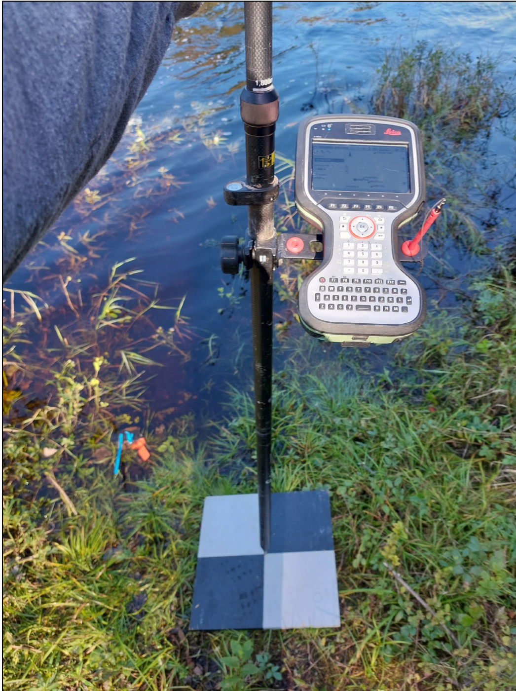
Figure 7. Using the Leica GS14 to collect a point for a ground truth location in Gold River on September 22 nd , 2023.
