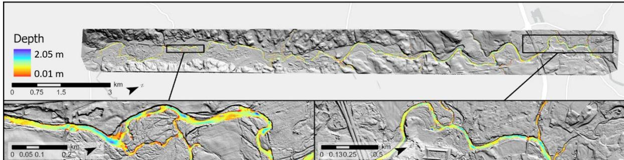
Figure 8. Depth map of River Philip captured during time of flight. The depth layer is overlaid on a hillshade of the digital elevation model.
