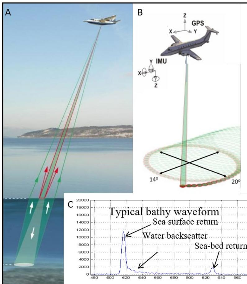
Figure 1. A) Interaction of the NIR and green laser light when travelling between air and water, refraction and scattering take place; B) Typical elliptical scan pattern for topo-bathymetric lidar with navigation system; C) Typical waveform captured from the green laser. Figure obtained from Leica, n.d.
