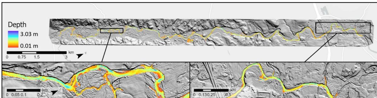
Figure 13. Modelled water depth of River Philip with a discharge value of  $13.63 \text{ m}^3/\text{s}$  set as a boundary condition.
