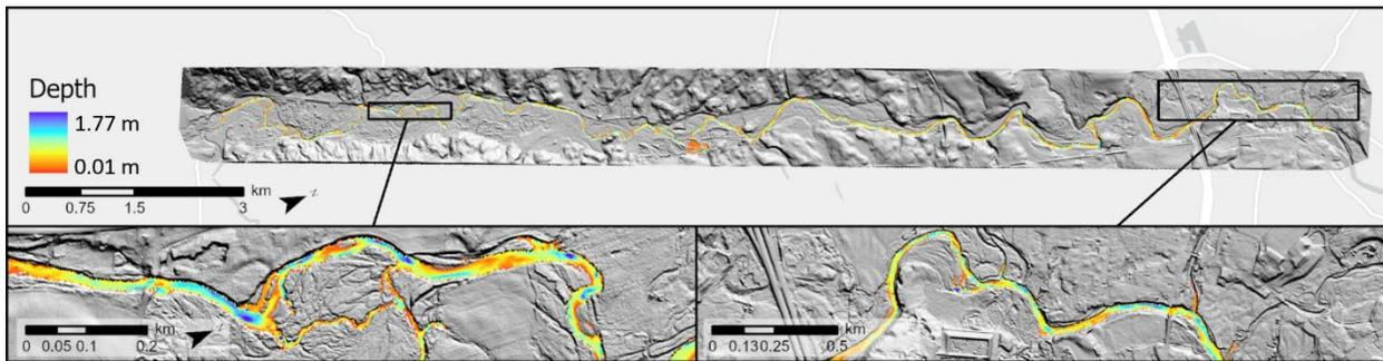
Figure 11. Modelled water depth of River Philip with a discharge value of  $3.95 \text{ m}^3/\text{s}$  set as a boundary condition.
