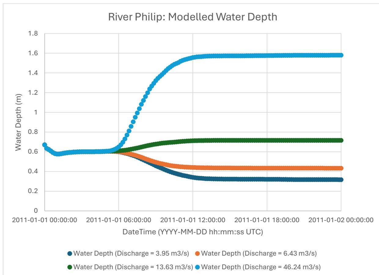
Figure 10. Water depths derived from the MIKE 21 hydrodynamic model at Water Street Bridge in Oxford, with different discharges set as boundary conditions within the model.
