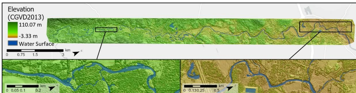
Figure 7. Digital surface model of River Philip displayed as a colour shaded relief with the water surface captured during the time of flight as an overlay.
