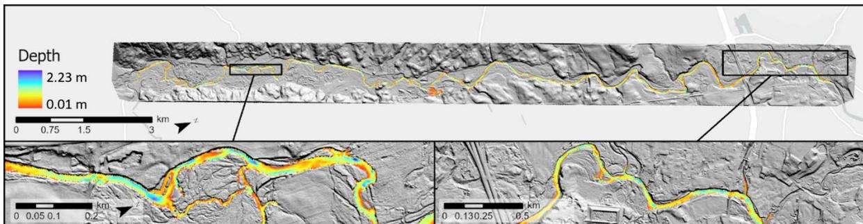
Figure 12. Modelled water depth of River Philip with a discharge value of  $6.43 \text{ m}^3/\text{s}$  set as a boundary condition.
