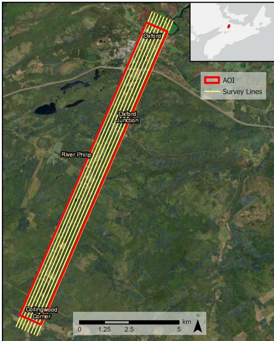
Figure 3. Extent of River Philip main stem surveyed with CH4X topo-bathymetric lidar scanner and RCD30 camera.
