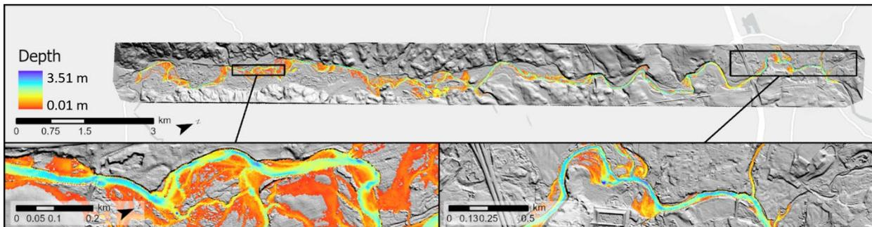
Figure 14. Modelled water depth of River Philip with a discharge value of  $46.24 \text{ m}^3/\text{s}$  set as a boundary condition.
