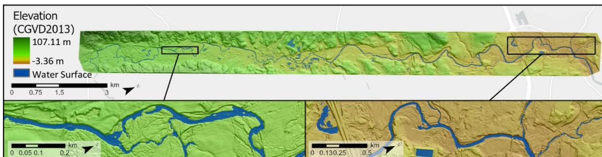
Figure 6. Digital elevation model of River Philip displayed as a colour shaded relief with the water surface captured during the time of flight as an overlay.
