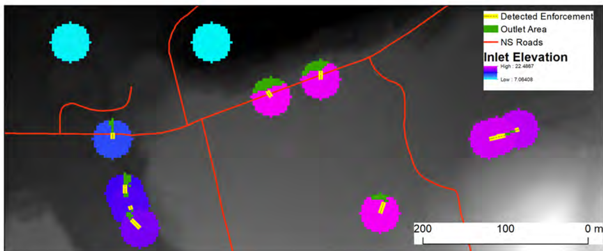
Figure 1.3 Example output from the custom enforcement (culvert) detection tool. Enforcement features identified as pools (center of circular buffer), where their elevation is compared to lowest neighboring DEM cells within 30 m (blue-pink elevation of the upstream buffer and green for downstream) a line feature (yellow) is constructed to the nearest lower cell.
