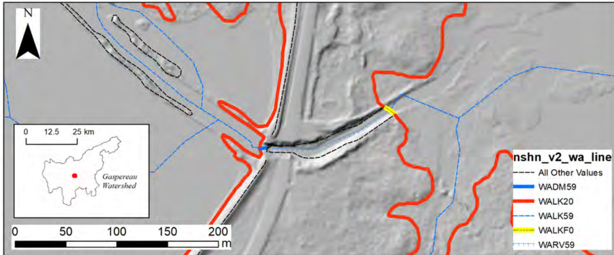
Figure 2.1 This figure shows Beaver Brook (Highway 12). Here we see that lake boundary (WALK20 in red) is depicted as a Barrier . This will ensure Channel features (blue) will be maintained where they intersect the lake features. Lake Delimiters (yellow) that do not act as barriers to imposing Channel features were unnecessary.
