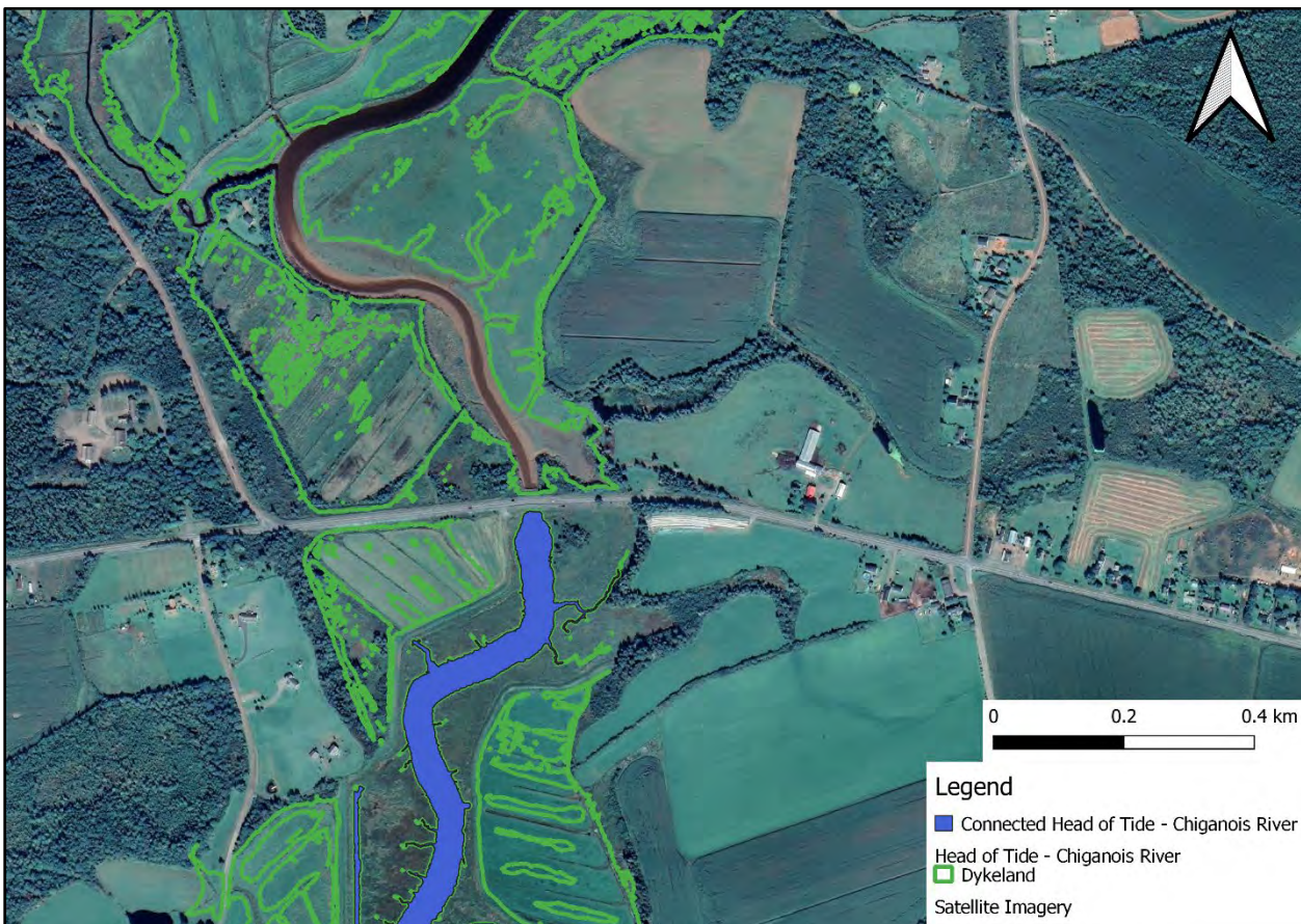
Figure 26 Example of a barrier (aboideaux) at Chiganois River that limits the head of tide for this river.
