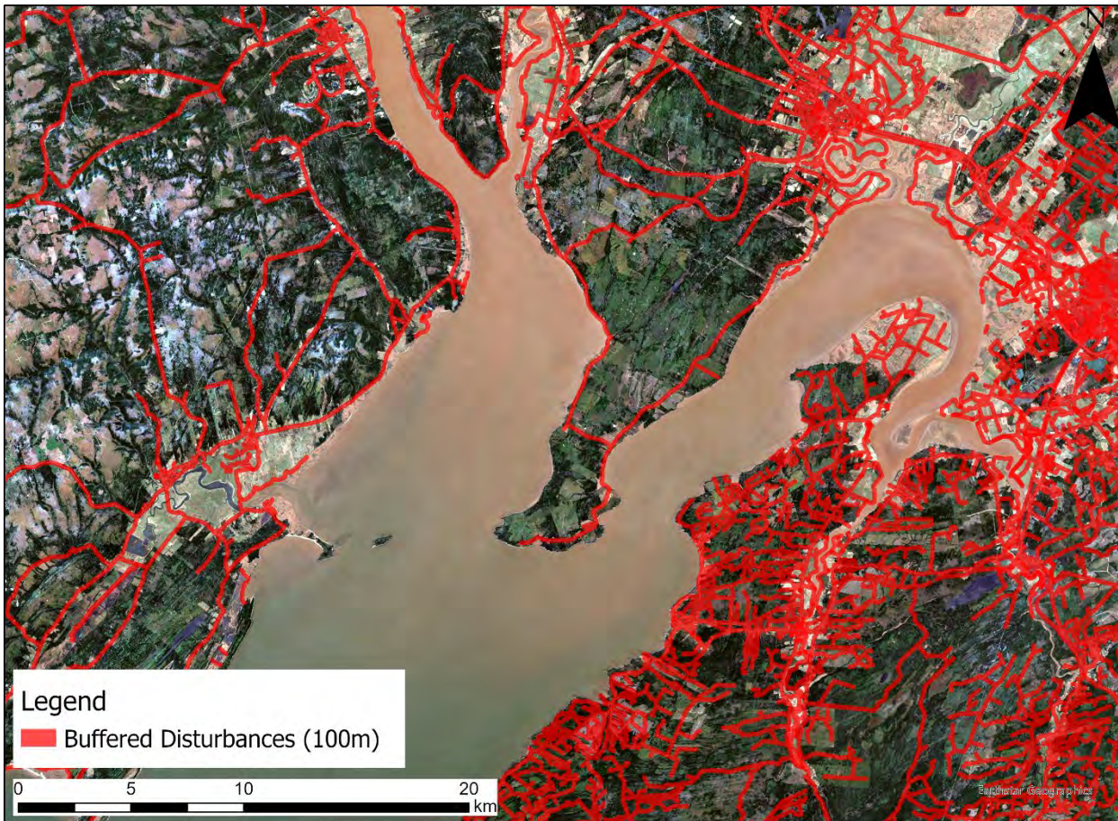
Figure 20 Example of 100 m buffer calculated for the road network, buildings and dykes in Chignecto Basin.
