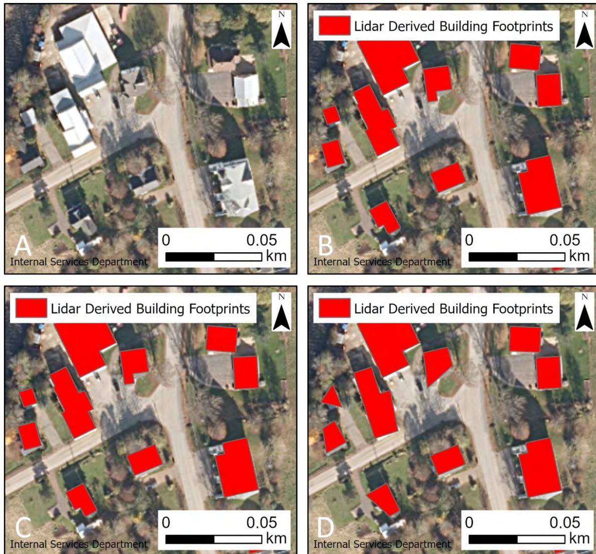
**Figure 25.** Maps showing a comparison between 2015 orthoimagery (A) and lidar-derived building footprints that have been regularized using right angles (B), right angles and diagonals (C), and any angle (D).
