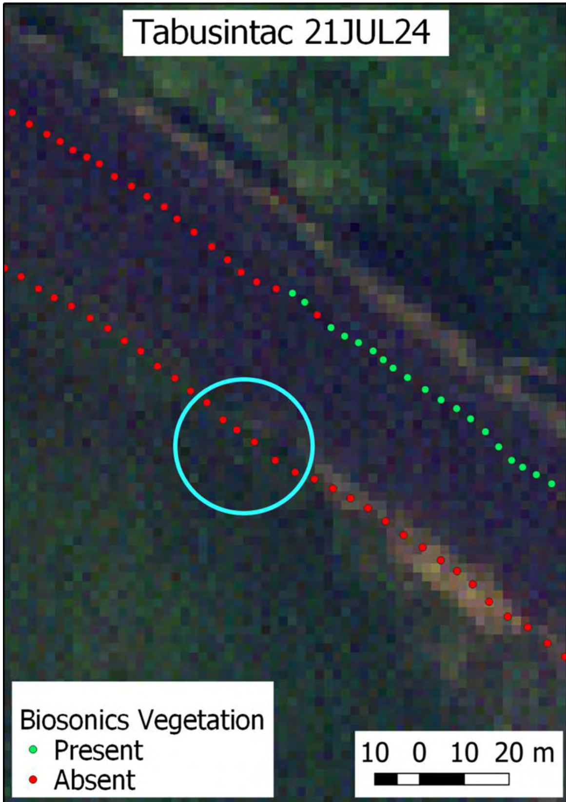
Figure 5 Inaccurate biosonics data collected in 2020 overlaid on a WorldView 2 image collected July 24th, 2021. The cyan circle outlines a few of these incorrect points, they are labeled as vegetation absent while located on top of eelgrass.
