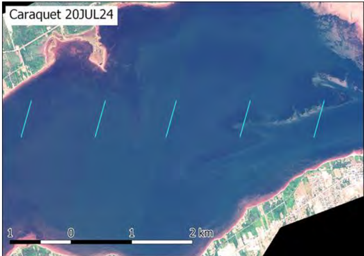
Figure 20 Vertical banding can be seen in the imagery, causing there to be lighter and darker areas in the image. The cyan lines are running partially along the boundaries of the banding artifacts and were added to help visualize their spacing.
