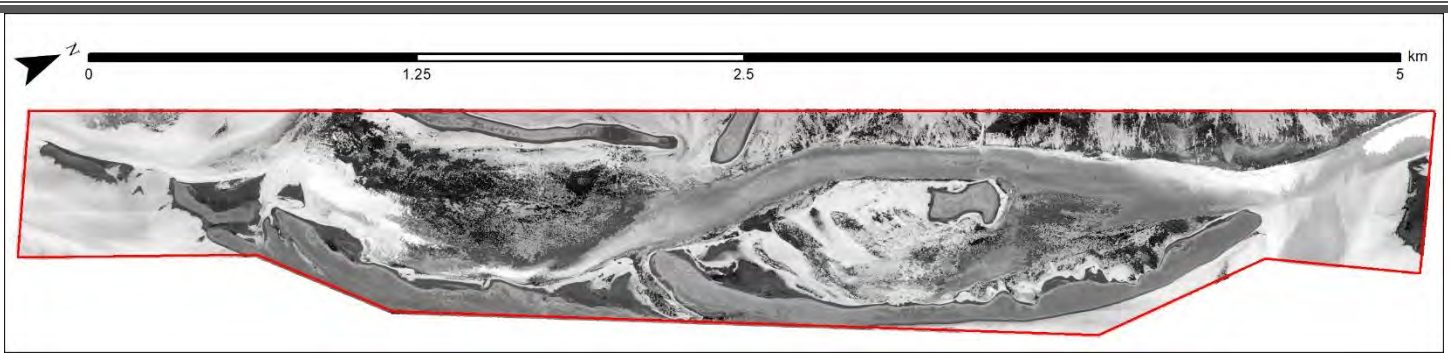
Figure 13. Depth normalized intensity map which separates highly absorbent materials, like eelgrass, from highly reflective materials, such as sand, regardless of depth.
