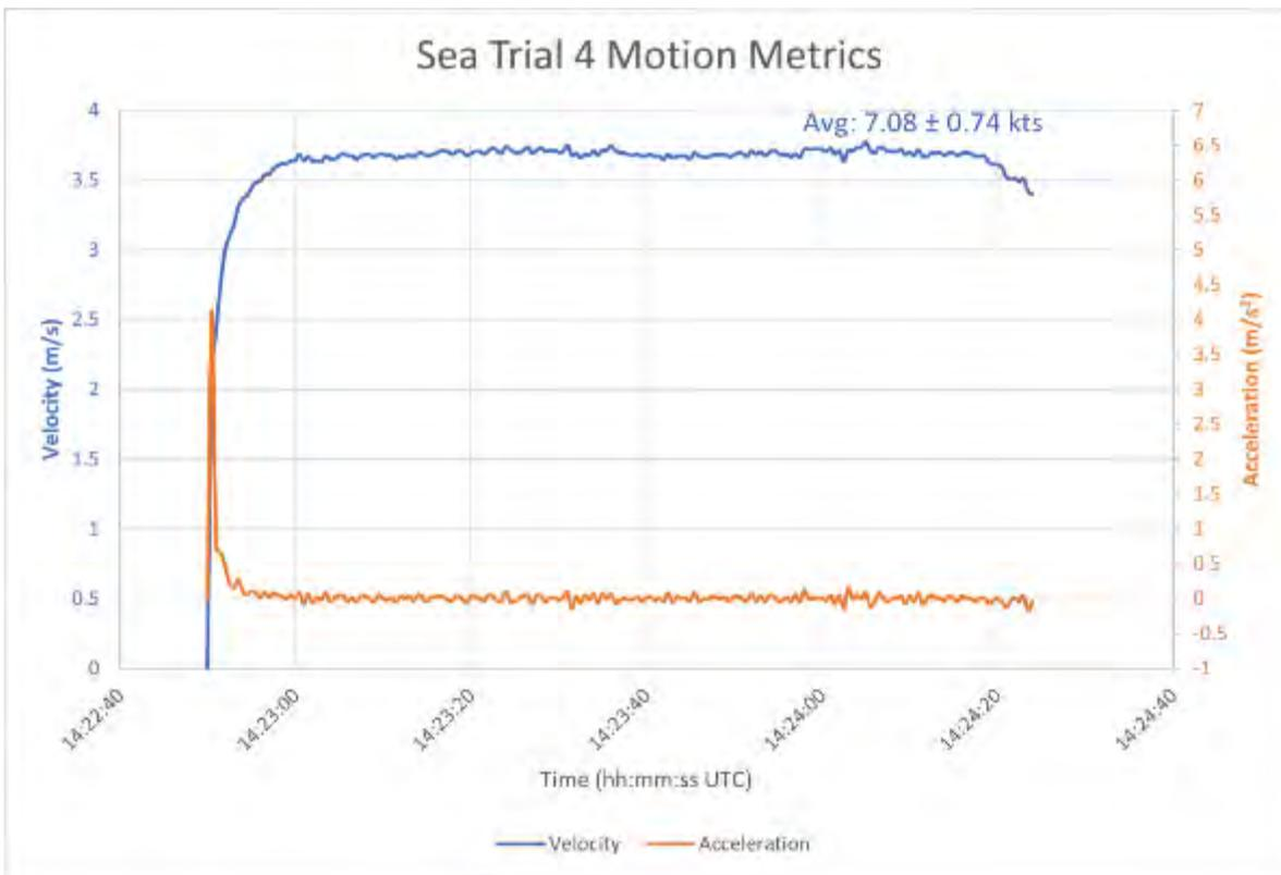
Figure 21. A graph of the velocity and acceleration calculated during the duration of the fourth sea trial.
