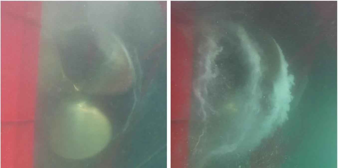
**Figure 25. The movement of the vortex cavitation is dependent on propeller direction: on the left the propeller is in reverse and the vortices are moving towards the prow, whereas on the right the propeller is in forward and the vortices move further away from the prow.**
