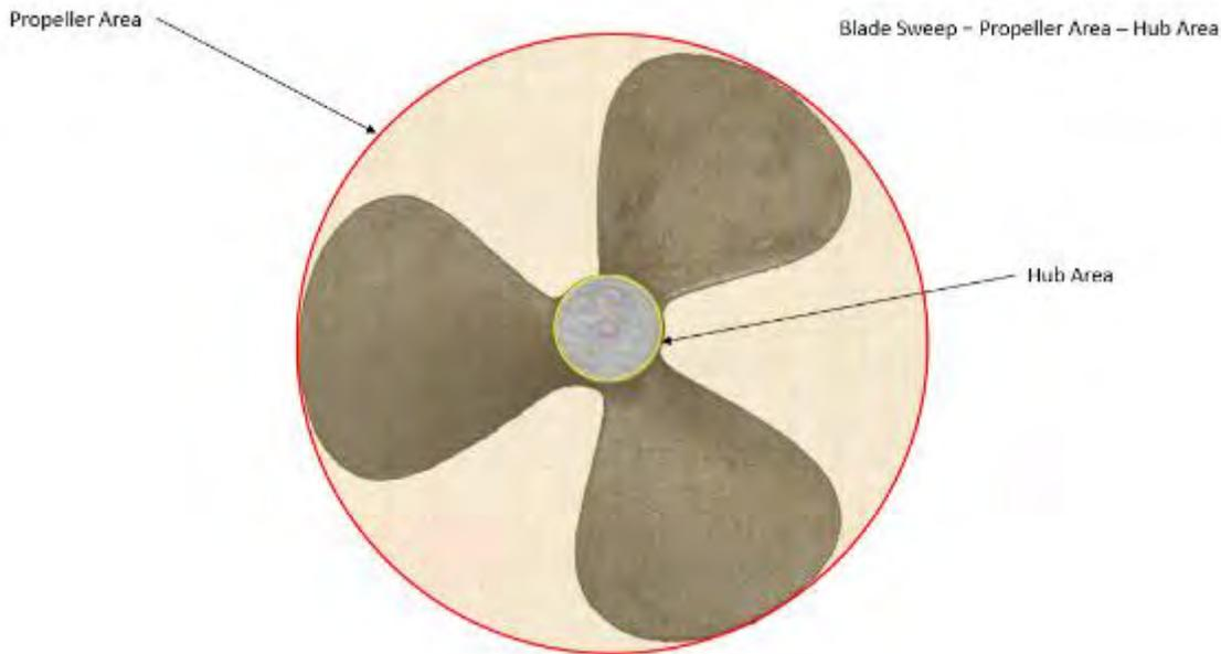
**Figure 7. A diagram showing how to calculate the blade sweep path area. The area of the total propeller area (red circle) is calculated, then the area of the propeller hub (yellow circle) is calculated. When you subtract the hub area from the total propeller area, the difference is the blade sweep path area.**
