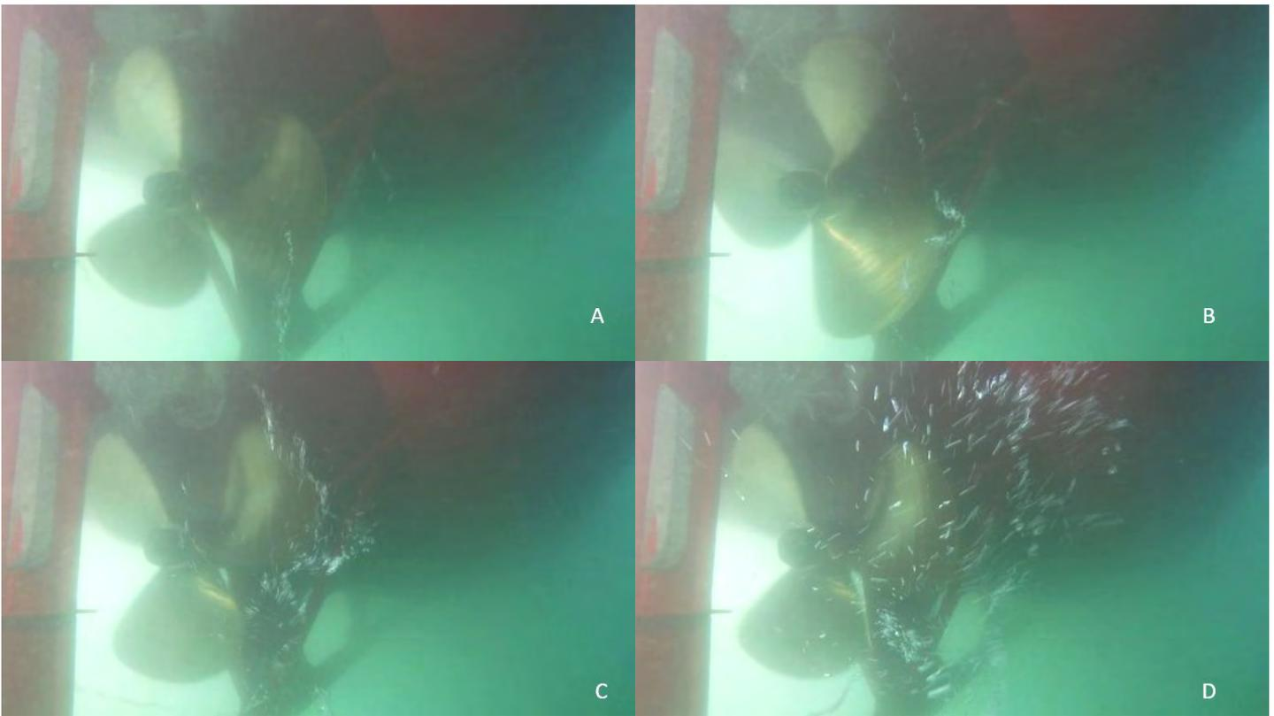
**Figure 31. A random chain of bubbles interacts with the propeller's water dynamic. A. A chain of bubbles enters the propeller area from below. B. The chain starts to twist as it encounters the water movement generated by the propeller blades. C. The chain is disrupted. D. The bubbles are flung violently out of the propeller area.**
