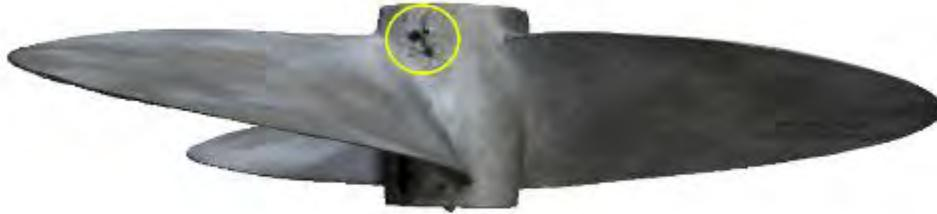
**Figure 28. A side view of the Grand Banks 3D model. A small hole is visible on the hub of the propeller.**
