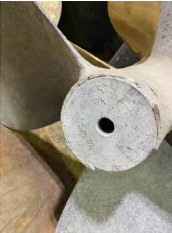
**Figure 2. A closeup of the hub of one of the propellers after it has been sprayed with the matte white formula and the black paint in preparation for being photographed and scanned.**
