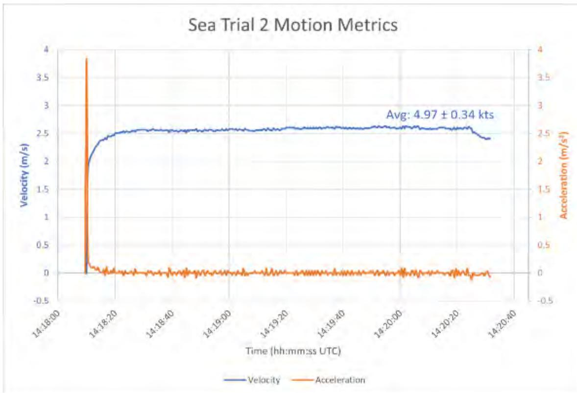
Figure 19. A graph of the velocity and acceleration calculated during the duration of the second sea trial.
