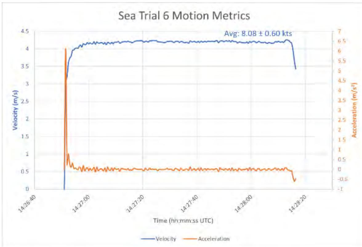
**Figure 23.** A graph of the velocity and acceleration calculated during the duration of the sixth sea trial.
