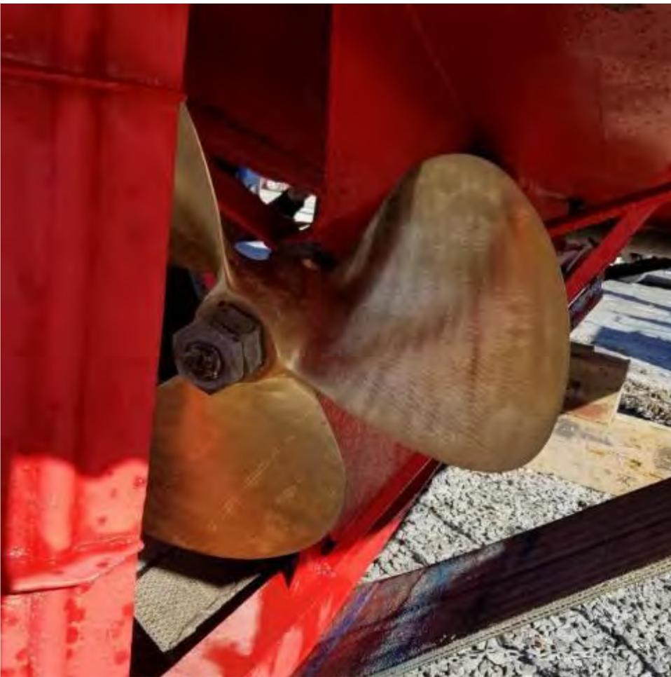
**Figure 8.** The Acadian propeller design by LIFE installed on their Mascot on the morning of the sea trials.
