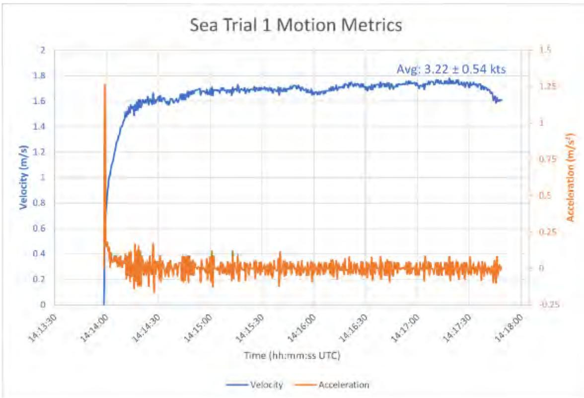
Figure 18. A graph of the velocity and acceleration calculated during the duration of the first sea trial.
