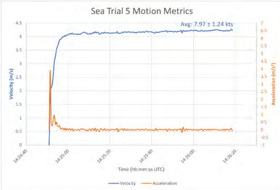
Figure 22. A graph of the velocity and acceleration calculated during the duration of the fifth sea trial.
