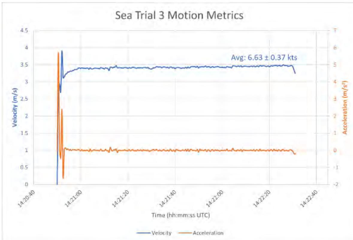
Figure 20. A graph of the velocity and acceleration calculated during the duration of the third sea trial.
