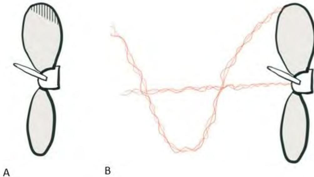
Figure 12. A diagram showing sheet cavitation (A) and vortex cavitation (B) (Cult of Sea, n.d.).
