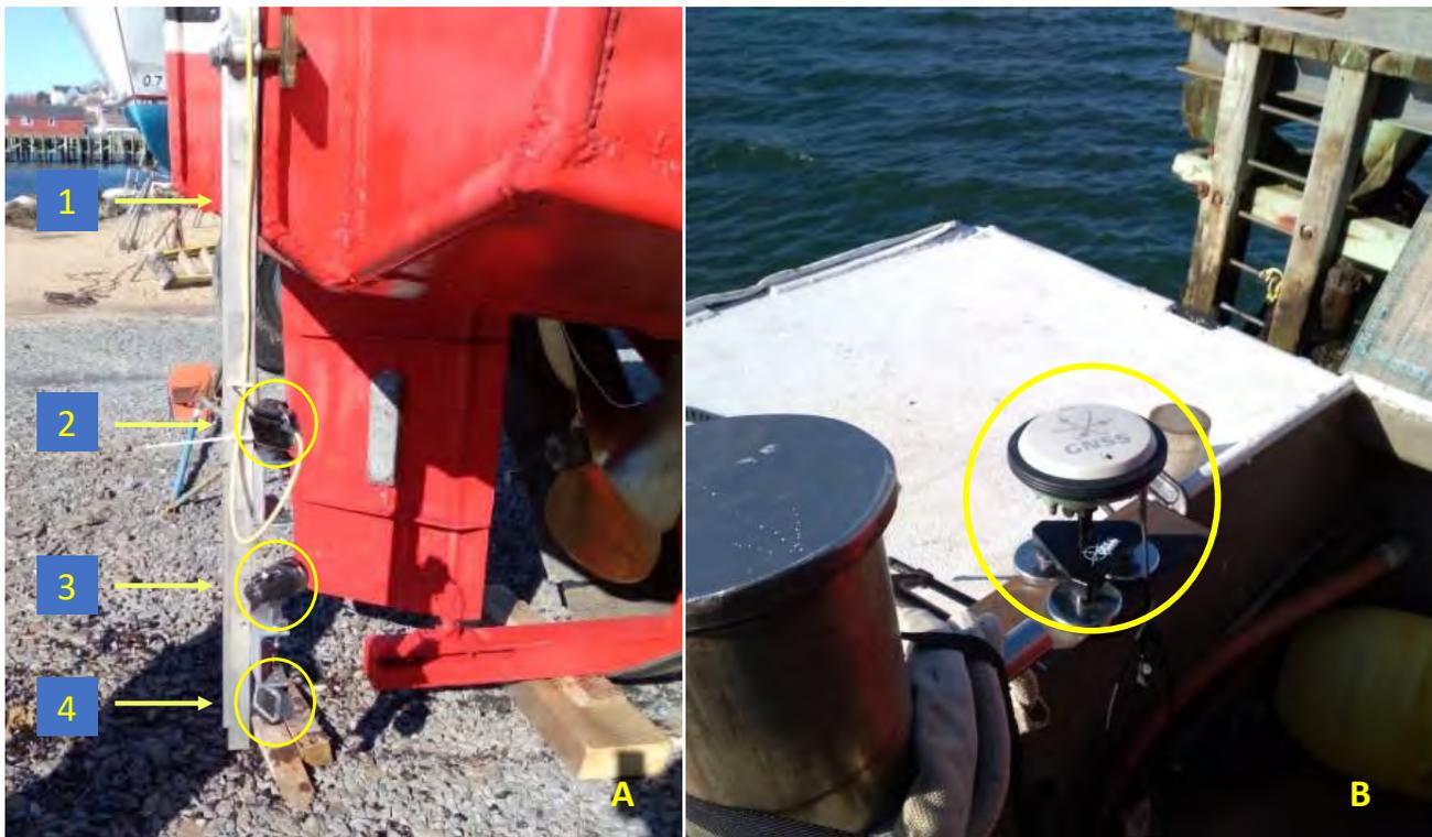
Figure 9. The equipment to capture data during the sea trials: A) mounted on a (1) custom designed strut off the stern: (2) a GoPro to capture still images; (3): a dive light to illuminate the propeller; (4) a GoPro to capture video and B) GNSS equipment mounted on the boat to collect survey quality positional data.
