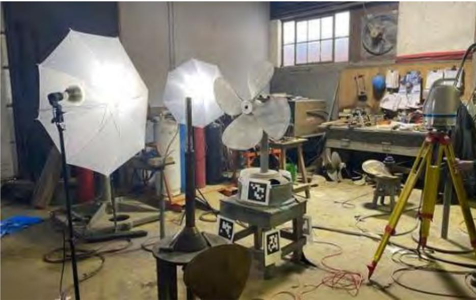
**Figure 4. The Bluenose propeller being laser scanned (scanner on tripod to the right).**
