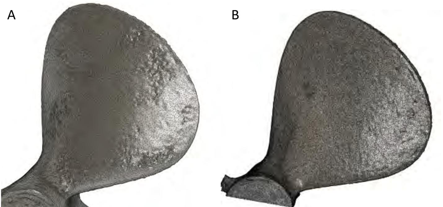
**Figure 27. Zoomed-in views of the back of the Acadian 3D model. A: The surface of one propeller blade shows a slight dimpling that may be erroneous. B: The surface of a different propeller blade is primarily smooth and shows little dimpling.**
