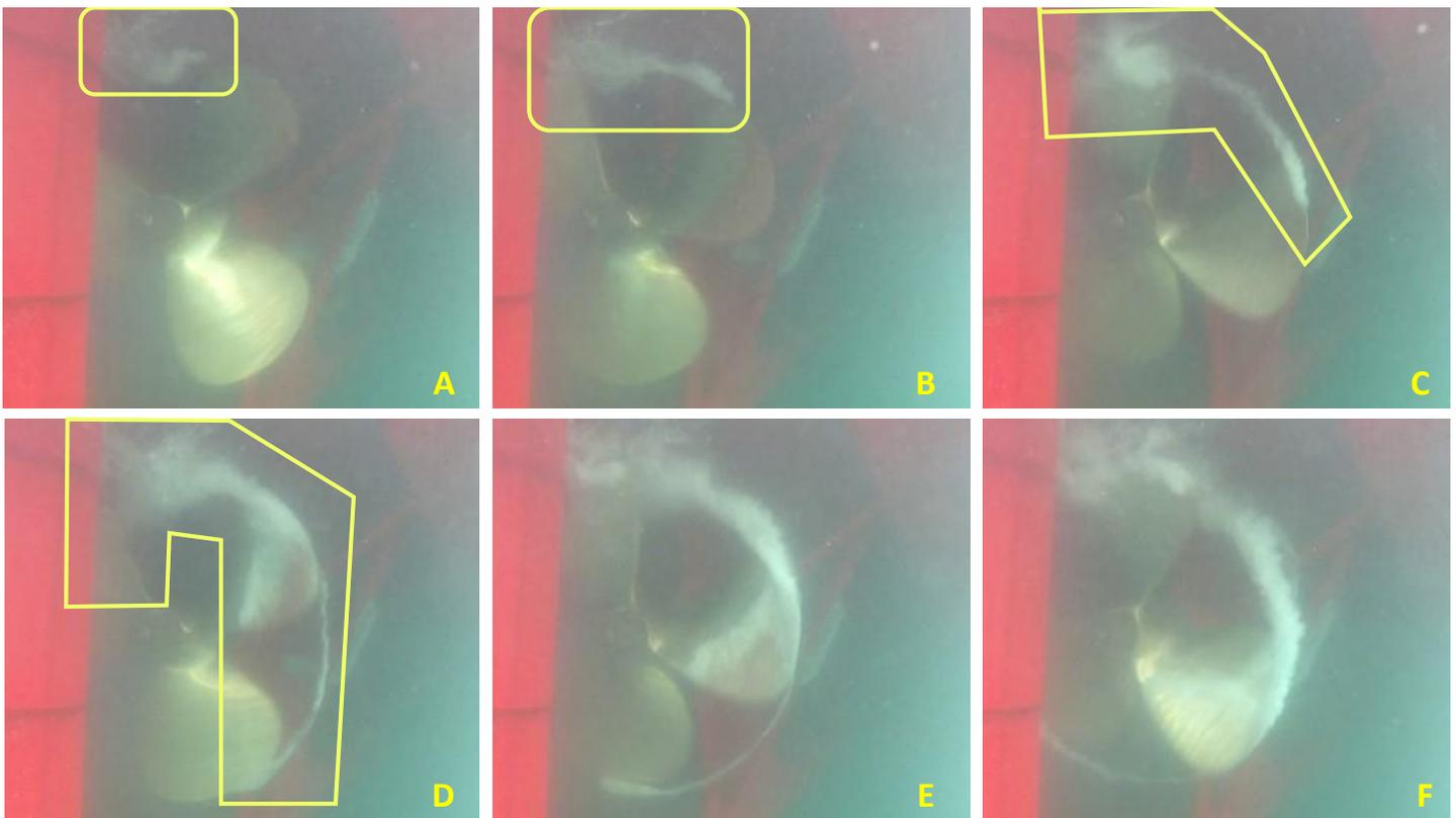
**Figure 24. The formation of a vortex cavitation spiral: A) bubbles forming a cluster between the top blades; B) the cluster is being stretched out into rope; C) the rope of bubbles is now following around blades and stretching along in an arc; and D – F) the bubble rope continues around the path of the blades, forming a ring around the propeller with foaminess still at top of blade area. (NB: images brightened by 20% from original)**
