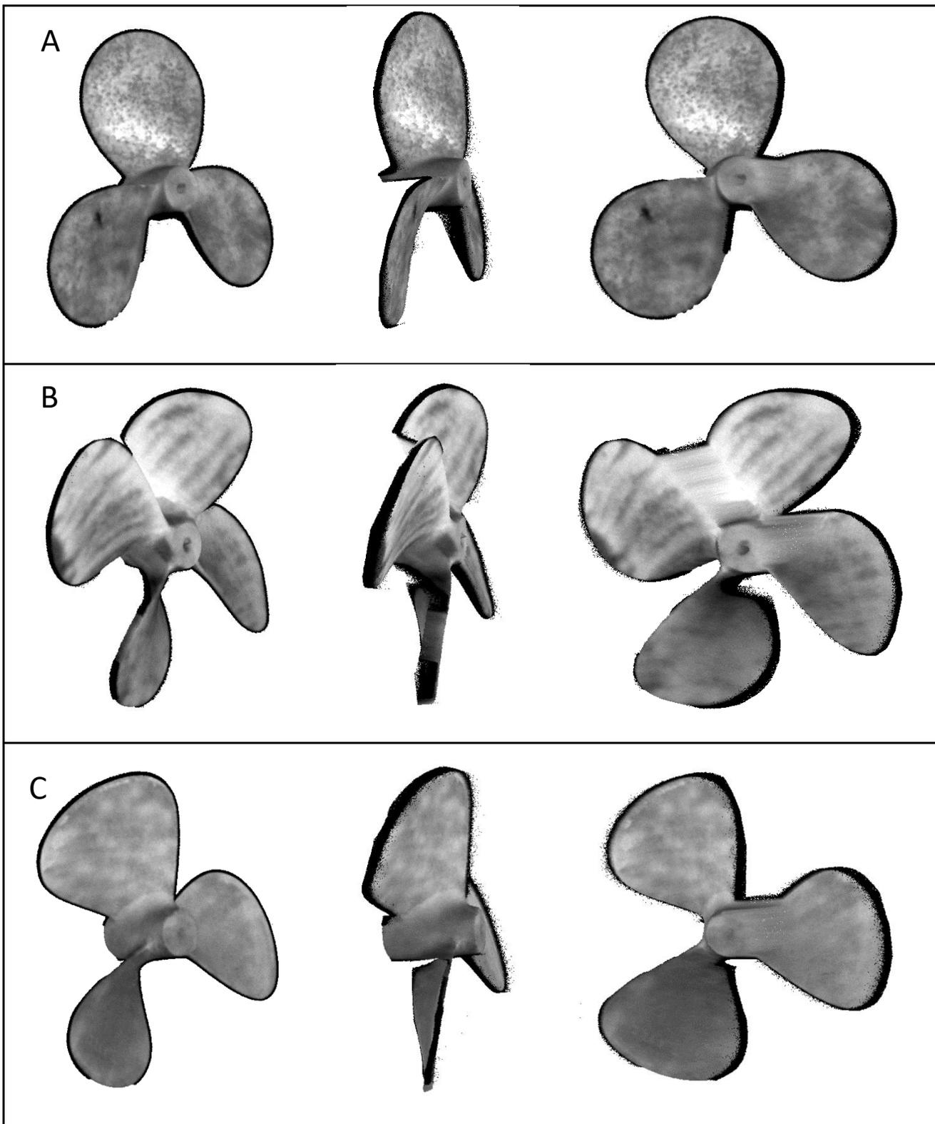
Figure 5. A point cloud taken with the Polaris terrestrial laser scanner from a single scan of the Grand Banks (A), Bluenose (B), and Acadian (C) propeller models. The left-most images show the propeller at the orientation in which it was scanned.
