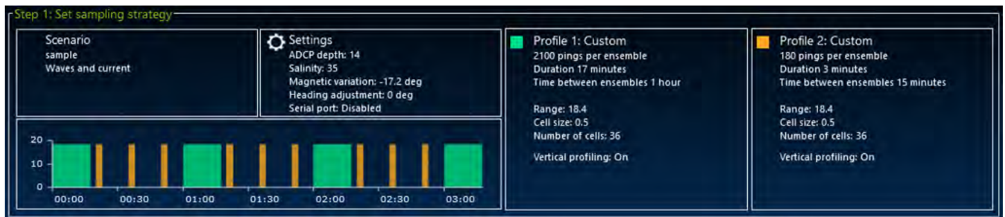
Figure 13 Setup of the Sentinel-V ADCP for waves and current measurement.
