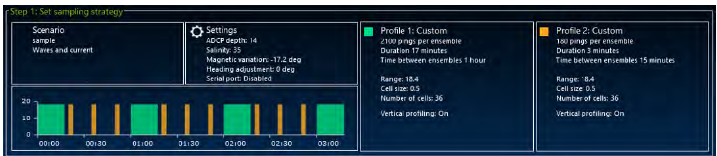
Figure 13 Setup of the Sentinel-V ADCP for waves and current measurement.
