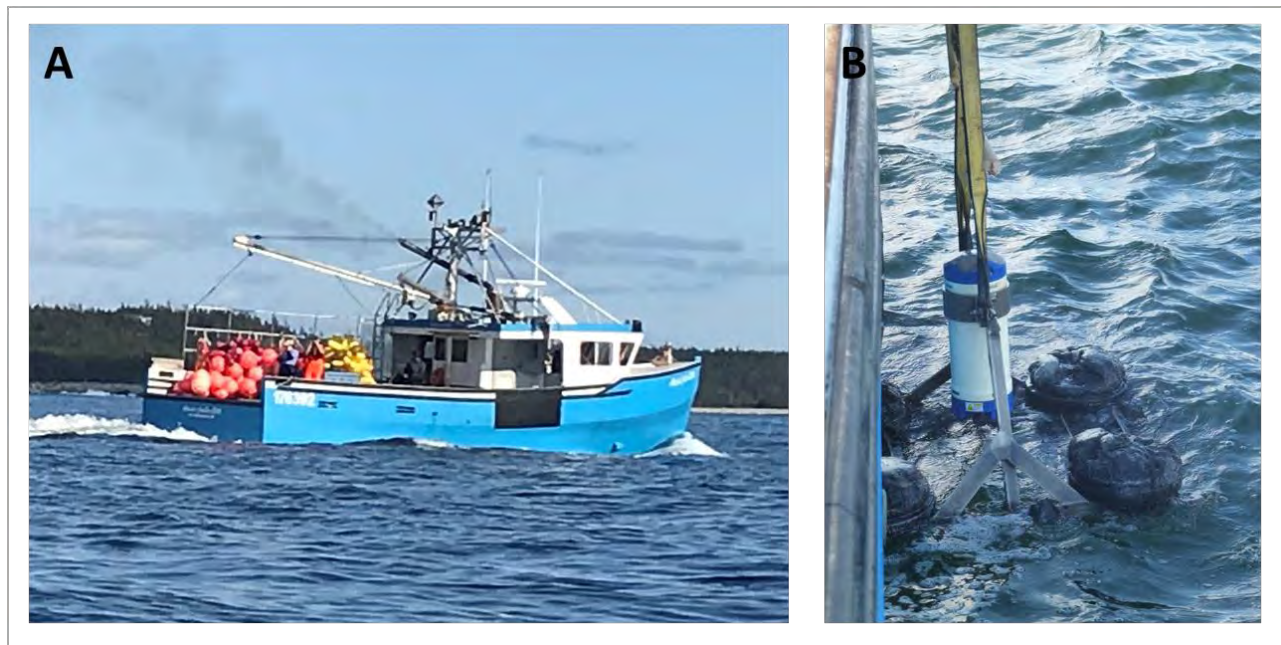
Figure 16 Retrieval of the ADCP from Indian Harbour. A- Fishing vessel Atlantic Crabber. B- ADCP being retrieved from the seabed along with the weights.
