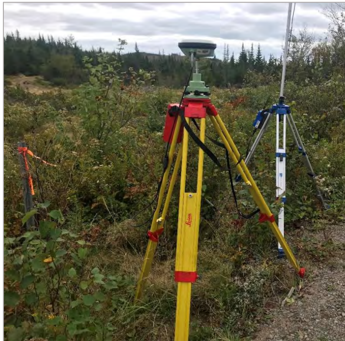
Figure 12 Base station set up on High Precision Network (HPN) station 210968 on Sonora road, to broadcast corrections using Pacific Crest ADL radio.
