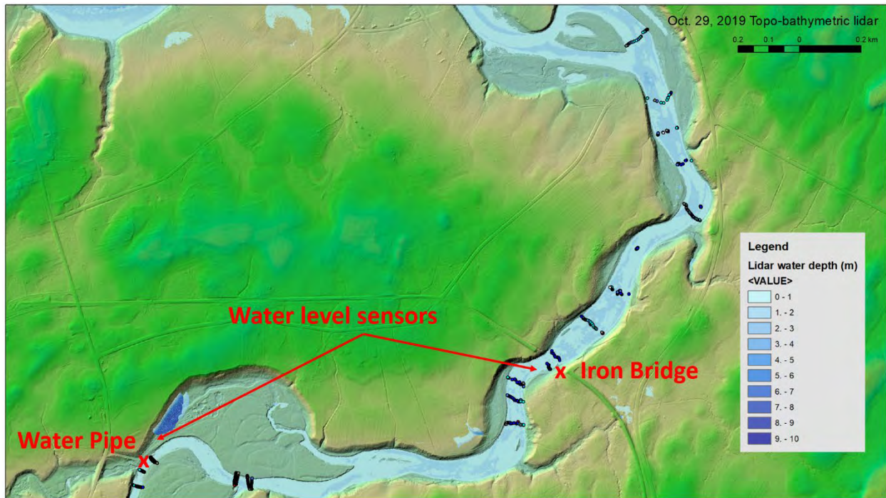
Figure 39 Water level sensors within River John at the "Iron Bridge" and the "Water Pipe" locations. The small dots represent river cross-section measurements.
