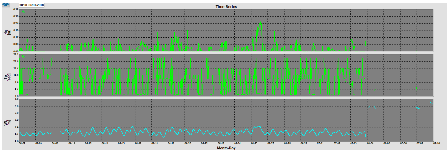
Figure 21: A plot showing the H_s (top graph), T_p (middle graph) and WL (bottom graph) during the ADCP deployment time frame.
