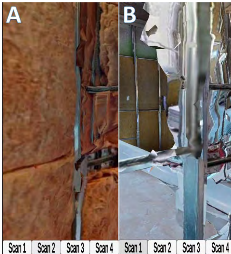
Figure 12 Side-by-side comparison of meshes of the same area from scan 2 (A) and scan 1 (B) taken from within the AR app.
