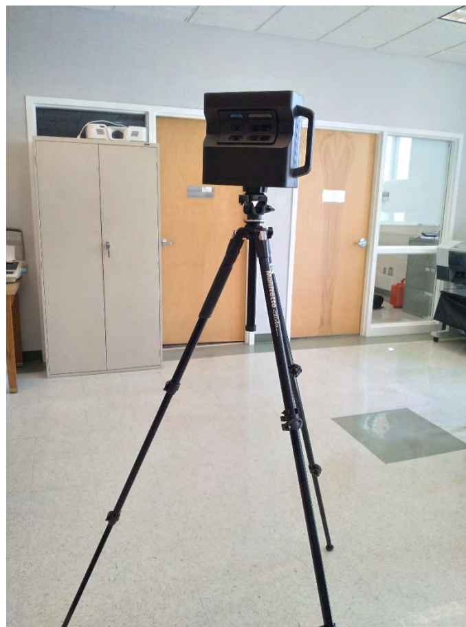
Figure 4 Matterport Pro installed on a tripod to conduct a 360° scan.
