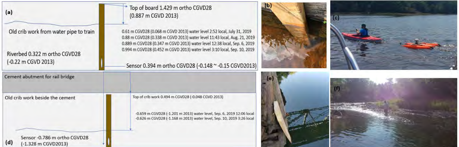
Figure 2.5 (a) Pressure sensor schematic upstream (b) Pressure sensor on a board attached to crib work near old water pipe (c) AGRG researchers conducting River Ray transect (d) Pressure sensor schematic downstream (e) Pressure sensor on a board attached to crib work to Iron bridge (f) Tim Webster collecting GPS transects.
