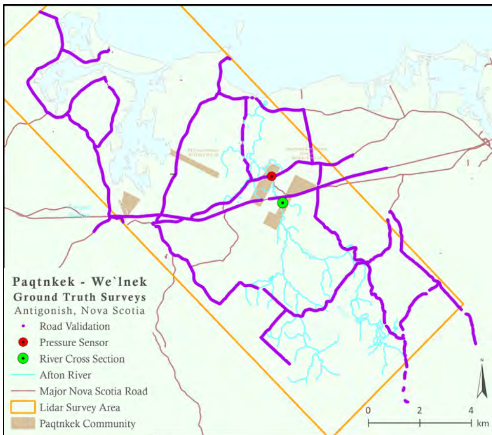
Figure 3.2: Lidar ground truth data collection for roads, cross sectional measurements for Afton River lidar validation to date, and location of pressure sensor in Afton River.
