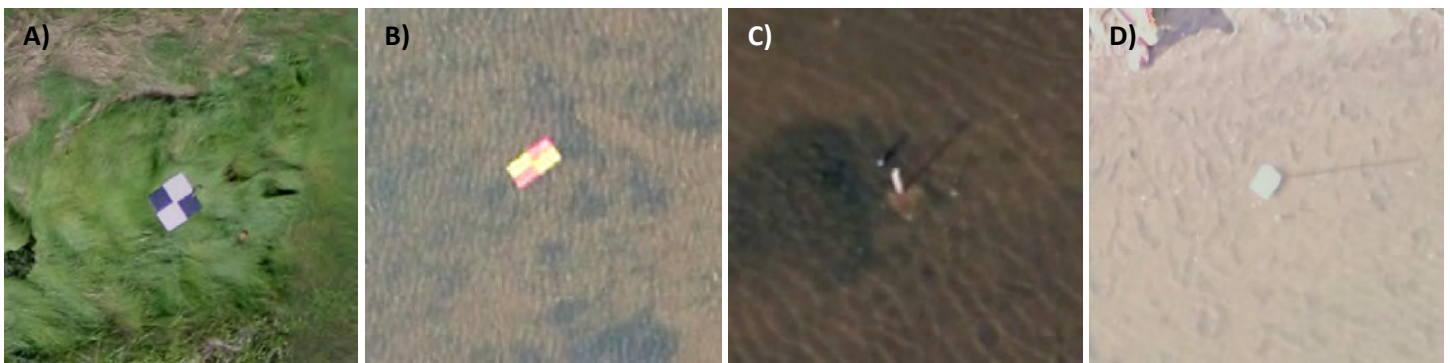
Figure 4.4: Examples of target visibility in multiple surveys. (A) Plywood photo target from Zenmuse X5 survey of Corduroy bed on Aug 10, 2018, 50 m altitude, 15 mm resolution. (B) Submerged cinder block target from Zenmuse X5 survey of Fireweed bed on Aug 10, 2018, 50 m altitude, 15 mm resolution. (C) Submerged cardboard target from Zenmuse X5 survey of Corduroy bed on Aug 10, 2018, 50 m altitude, 15 mm resolution. (D) Floating cardboard target from Zenmuse X5 survey of Fireweed bed on Aug 10, 2018, 50 m altitude, 15 mm resolution.
