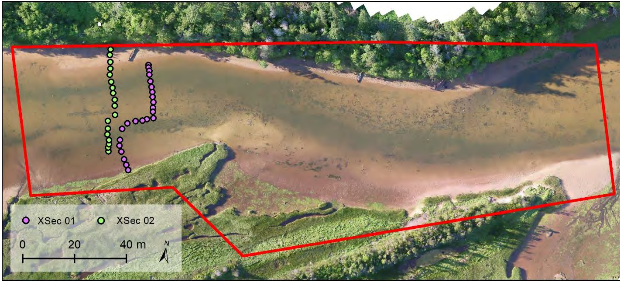
Figure 3.11: Location of PPK GPS point cross sections collected in Main bed on Aug 11, 2018.
