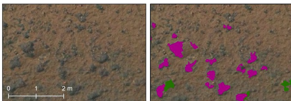
Figure 3.19: Classification of 10 mm orthomosaic and elevation model (RGB, NHM) using an object-based classification in eCognition. Survey was completed with the Mavic camera on August 11, 2018 at 19:06 (ADT) during a rising mid tide with a flight altitude of 30 meters. Red polygon represents Main Bed study area boundaries, black polygons represent subsequent close-ups of the imagery/classification.
